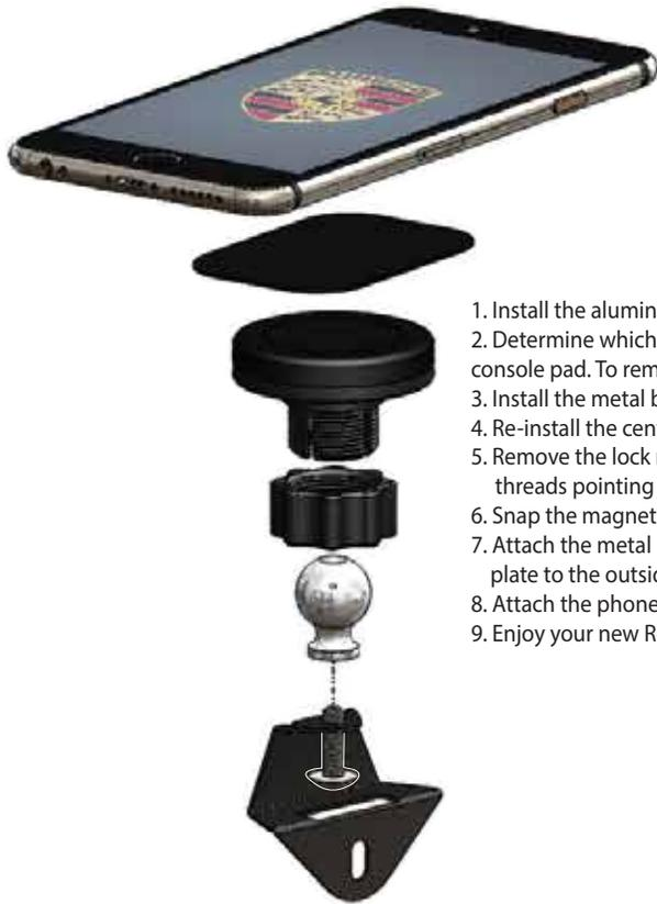
1. Install the aluminum ball onto the metal bracket as shown using the supplied screw.
